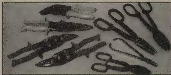
Above: Snips and shears commonly used for cutting tin. Note the compound hinges on the
